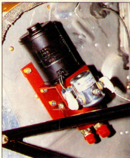
To improve safety and reliability, we added an Oilamatic Preoiler (above) and a Precise Flight standby vacuum system. The Oilamatic eases starting wear and tear; the Precise Flight does the same for the pilot if the vacuum pump fails.
